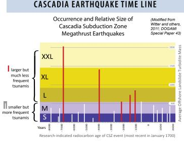
Average offshore landslide turbidite mass is used as a proxy for earthquake size.
